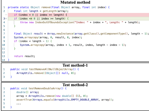
Figure 1: Motivating example of two mutant-test pairs formed by the same mutant with two tests from the commons-lang project (commit d1a45e9). The mutated line is highlighted with color (i.e., the line is mutated from the red line to the green line). Test method-2 kills the mutant (i.e., detects the changed behavior) while Test method-1 does not.
